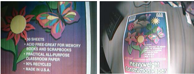
Figure 4. Images obtained from our camera’s default narrow-angle lens (left) and the fisheye lens that we installed (right).
